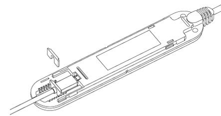
4. Remove the micro USB-B cable from Pronto and replace it with the alternative micro USB-B cable that has a USB-A connector at the other end.
